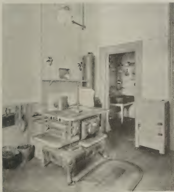
THIS SHOWS WHAT TO AVOID. THE ICE BOX IS TOO NEAR THE STOVE. COAL SHOULD BE KEPT IN ONE RECEPTACLE. THE SINK IS IN A DARK CORNER. THE TOWELS ARE AT THE STOVE WHERE THEY MAY CATCH FIRE INSTEAD OF AT THE SINK WHERE THEY ARE NEEDED
